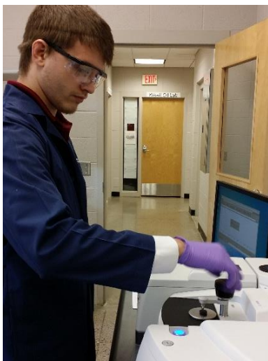
Figure 1. Validation of compounds in the product using FTIR-ATR.
